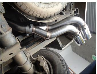
**Step 6.** Next, loosely slip the Hanger Clamp Assembly over the Tail Pipe Assembly and Install using the supplied clamps and by fitting the welded hangers into the rubber insulators.
